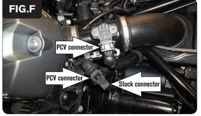
10 Plug the pair of 3-pin PCV leads in-line of the bike's Throttle Position Sensor and the stock wiring harness (Fig. F).
