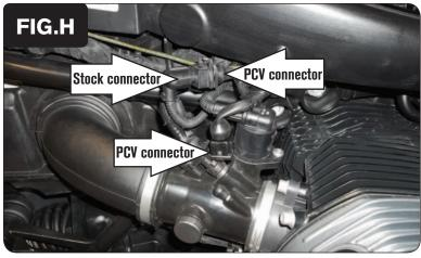
Plug the pair of PCV leads with YELLOW colored wires in-line of the right side Fuel Injector and the stock wiring harness.
