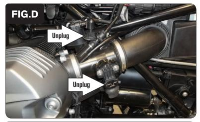
At the left side throttle body, unplug the fuel injector and unplug the Throttle Position Sensor (Fig. D).
