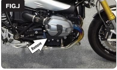
Remove the small plastic panels beneath the cylinder heads on both sides of the bike (Fig. J).
